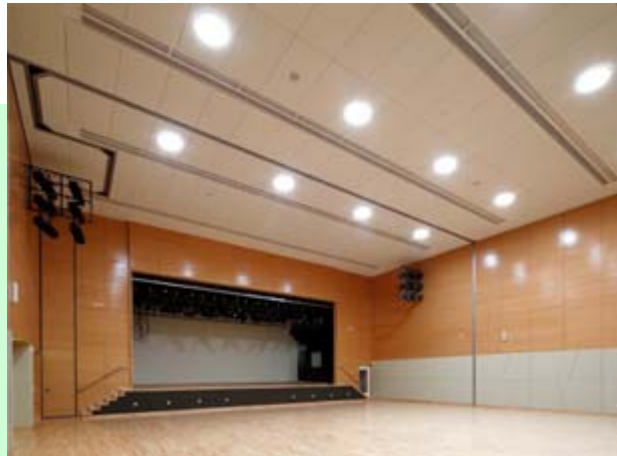
Sun pipes transmit sunlight from the roof of the community hall (left) through high reflective internal surfaces to the multi-purpose hall (right)
