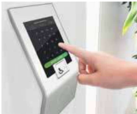
(e) Destination control panel
