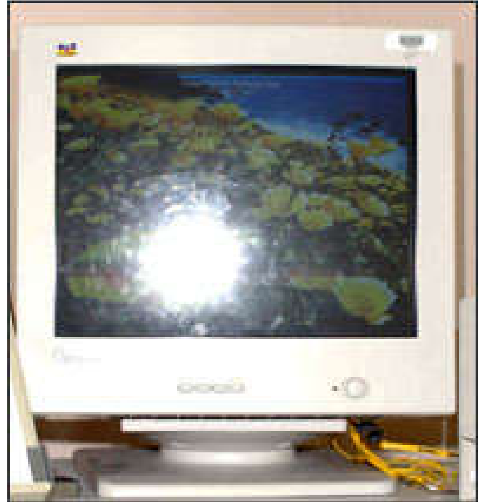
Veiling reflection from overhead light source
