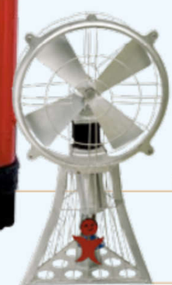
煤氣風扇 Gas-powered fan
