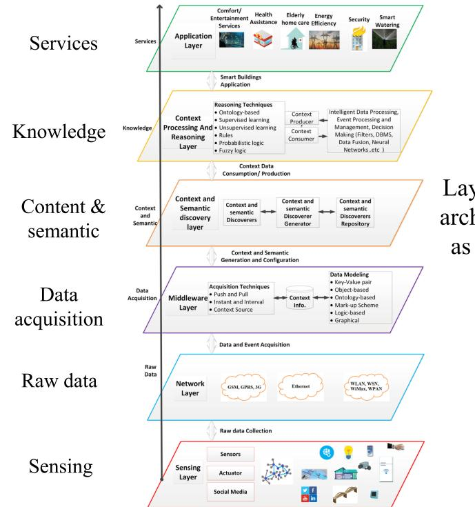
Layers of the base IoT architecture that serves as the foundation for smart buildings
