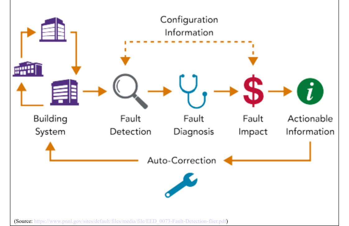
Common measures identified & implemented through use of automatic fault detection & diagnostics (AFDD) technology
