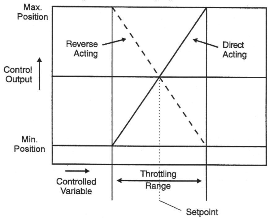
[Source: Honeywell, 1997. Engineering Manual of Automatic Control for Commercial Buildings]
