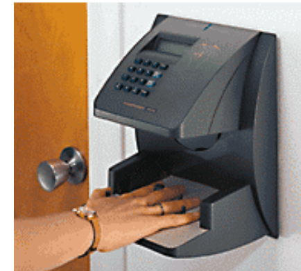
Access Control Terminal
