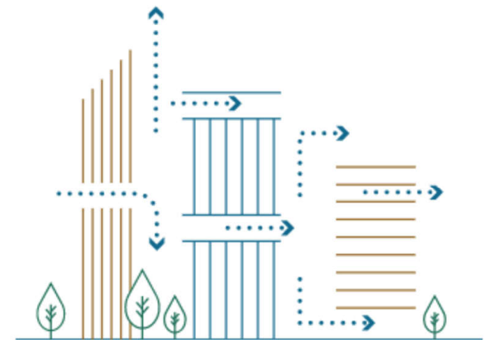
Air ventilation around buildings
