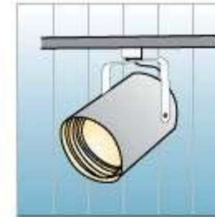
Track Lighting (Incandescent)
