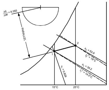
The above figure shows the schematic solution. State 2 is located on the ASHRAE chart. From thermodynamic properties table, the specific enthalpy of the added water vapor is hg = 2555.58 kJ/kg. From the psychrometric equation,
