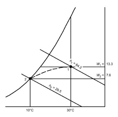
The above figure shows the schematic solution. State 1 is located at the intersection of  $t = 30^{\circ}\text{C}$  and  $\phi = 50\%$ . Thus,  $h_1 = 64.3$  kJ/kg (dry air),  $W_1 = 13.3$  g (water)/kg (dry air), and  $v_1 = 0.877$  m<sup>3</sup>/kg (dry air). State 2 is located on the saturation curve at 10°C. Thus,  $h_2 = 29.5$  kJ/kg (dry air) and  $W_2 = 7.66$  g (water)/kg (dry air). Given:  $h_{w2} = 42.11$  kJ/kg (water). The mass flow of dry air is:
