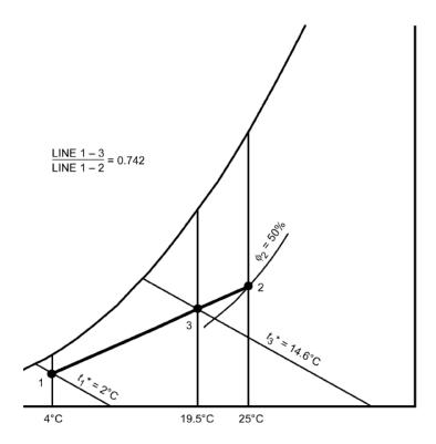
The above figure shows the schematic solution. States 1 and 2 are located on the ASHRAE chart, revealing that  $v_1 = 0.789 \text{ m}3/\text{kg}$  (dry air), and  $v_2 = 0.858 \text{ m}^3/\text{kg}$  (dry air). Therefore,
