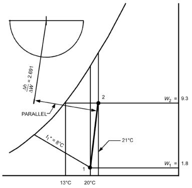
The above figure shows the schematic solution. From a steam properties table, the enthalpy of the steam  $h_g = 2691$  kJ/kg (water). Therefore, according to the psychrometric equation, the condition line on the psychrometric chart connecting States 1 and 2 must have a direction:
