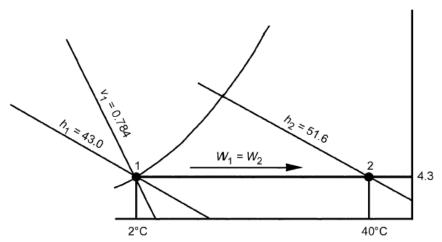
The above figure schematically shows the solution. State 1 is located on the saturation curve at 2°C. Thus,  $h_1 = 13.0 \text{ kJ/kg}$  (dry air),  $W_1 = 4.3 \text{ g}$  (water)/kg (dry air), and  $v_1 = 0.784 \text{ m}^3/\text{kg}$  (dry air). State 2 is located at the intersection of t = 40°C and  $W_2 = W_1 = 4.3 \text{ g}$  (water)/kg (dry air). Thus,  $h_2 = 51.6 \text{ kJ/kg}$  (dry air). The mass flow of dry air is:
