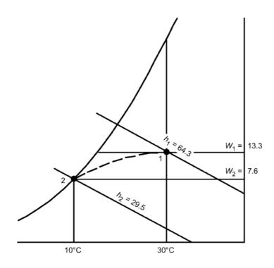
The above figure shows the schematic solution. State 1 is located at the intersection of  $t = 30^{\circ}$ C and  $\varphi = 50\%$ . Thus,  $h_1 = 64.3$  kJ/kg (dry air),  $W_1 = 13.3$  g (water)/kg (dry air), and  $v_1 = 0.877$  m<sup>3</sup>/kg (dry air). State 2 is located on the saturation curve at 10°C. Thus,  $h_2 = 29.5$  kJ/kg (dry air) and  $W_2 = 7.66$  g (water)/kg (dry air). Given:  $h_{w2} = 42.11$  kJ/kg (water). The mass flow of dry air is:
