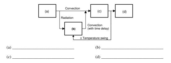
10. The diagram below shows the solar heat gain and cooling load curves at a west window of a building. Fill in the blanks below for the elements represented by (a) to (d) in the diagram.
