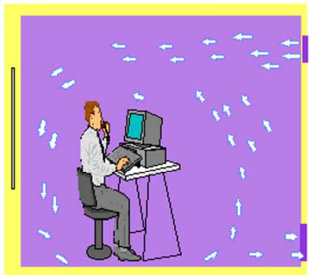
Mixing ventilation (MV)
