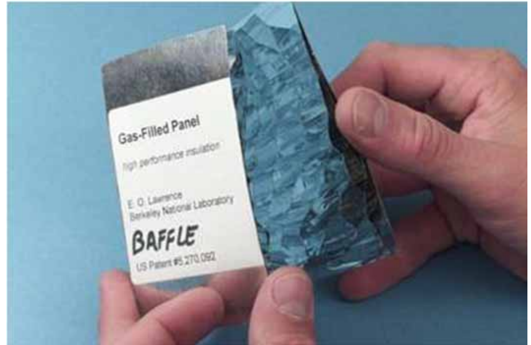
Gas filled panel (high performance insulation)
