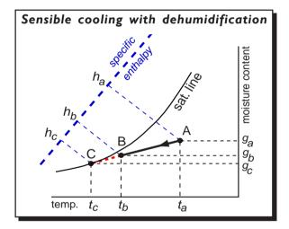
Thus there will be both a reduction in temperature and a reduction in moisture content and condensation will occur on the cooling coil surface.
