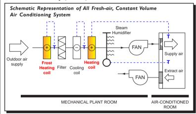
An air heater battery (or coil) normally comprises of a number of heating elements, arranged at right angles to the directio of air flow, contained within a sheet metal casing with flanged ends. The heating elements are either plain or finned tubes, carrying water or steam, or electric heating elements. Steam tubes (always) and electric elements (usually) are arranged vertically and hot water tubes horizontally. Tubes are of copper with either copper or aluminium fins.
