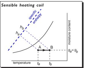
If air at condition A is heated to condition B, it will increase in dry-bulb temperature but the moisture content will remain constant. The enthalpy will increase and all the increase will be sensible heat (i.e. heat causing a temperature rise).
