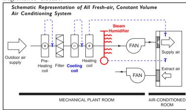
In some instances, particularly industrial applications requiring high humidity **Direct Humidification** is used. This can be achieved using water which can be "atomised", either by injecting with compressed air through high pressure nozzles, or mechanical impingement. Alternatively steam can be injected directly into the space.
