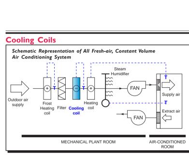
Air cooling coils (or batteries) are similar to air heaters with the additional provision of a collection tray and drain for condensate.
