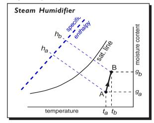
It should be noted that effectiveness does not apply to either steam or direct water injection humidifiers. It is possible to supply too much steam to an air stream in which case "fogging" will occur and some form of safeguard is usually fitted to prevent this.
