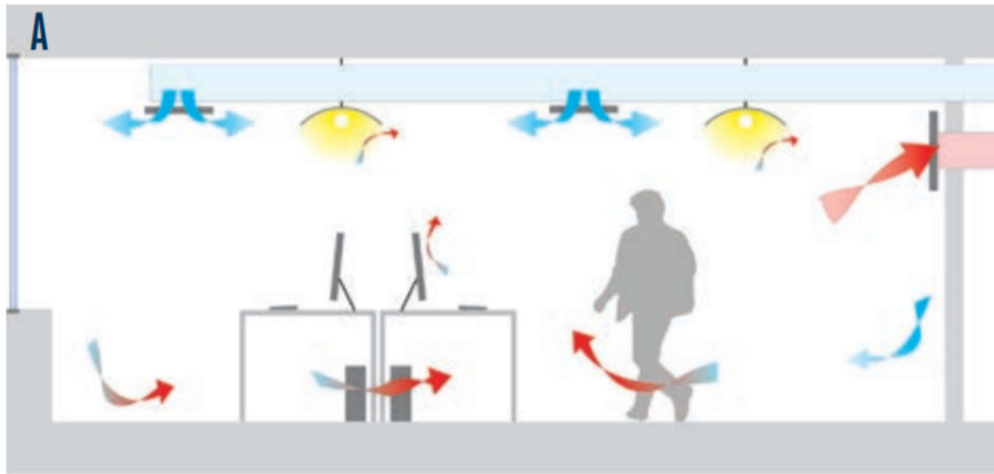
Overhead air distribution system
