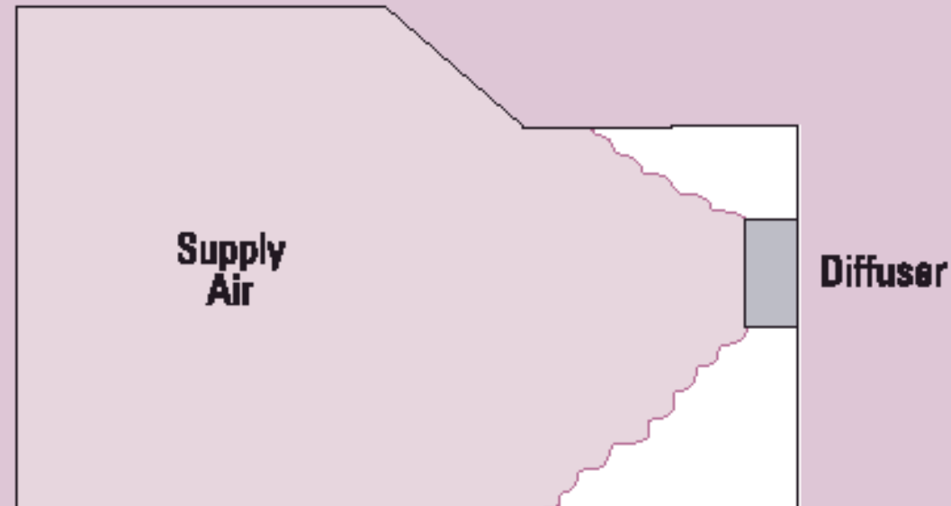
Figure 8 - Irregular Room Geometry
