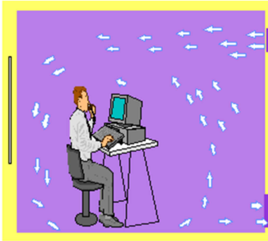
Mixing ventilation (MV)
