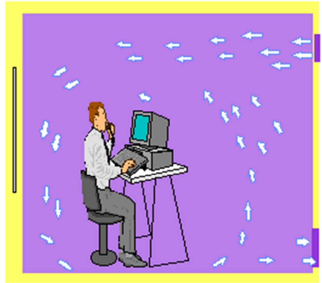
Mixing ventilation (MV)
