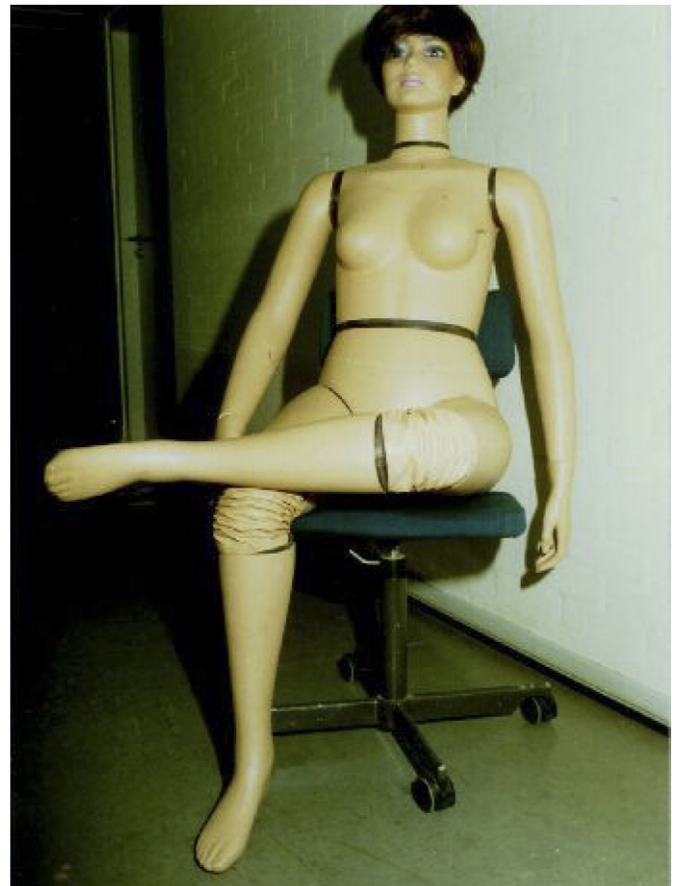
Fig. 1. The manikin (divided into 20 independent segments, each with its own heating and computer control system).
