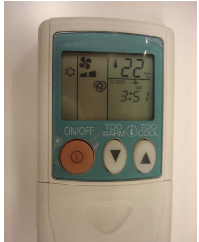
Fig. 7. The remote controller of a typical SRAC showing indoor air temperature setting.
