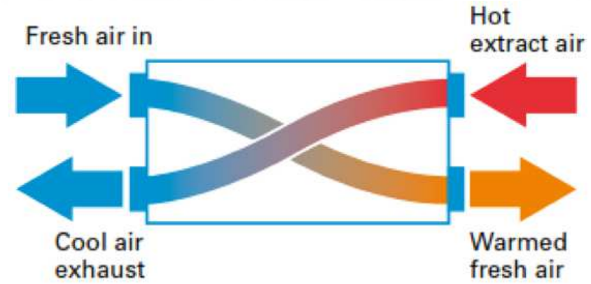
Figure 8.19 Schematic winter air conditioning system using 100 percent outdoor air with preheating by waste heat from the exhaust air.
