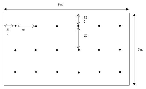
Therefore in this example the spacing between points along rows along the length of the interior  $= 9 \div 6 = 1.5$ m and the distance of the 'end' points from the wall  $= 1.5 \div 2 = 0.75$ m.
