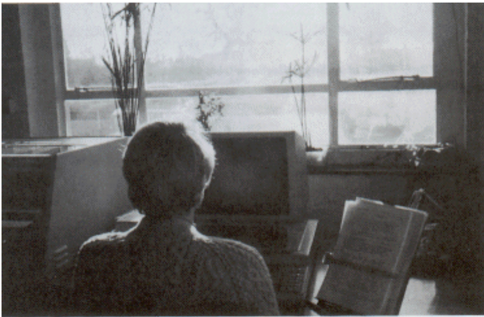
Disability glare from bright sky in front of a VDT makes the screen difficult to read
