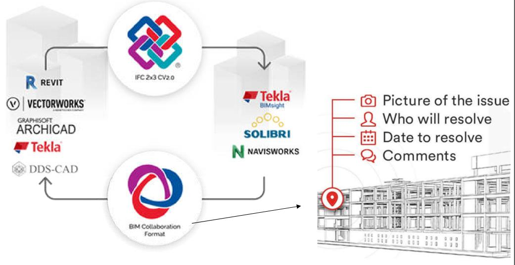
BCF is the communication between IFC tools and native modelling software. The BCF will identify exactly which objects are involved in an issue and will even record the screen view. So, when someone opens up a BCF issue in their modelling software they are directed to the exact same view in their model.
