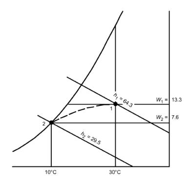
The above figure shows the schematic solution. State 1 is located at the intersection of  $t = 30^{\circ}$ C and  $\varphi = 50\%$ . Thus,  $h_1 = 64.3$  kJ/kg (dry air),  $W_1 = 13.3$  g (water)/kg (dry air), and  $v_1 = 0.877$  m<sup>3</sup>/kg (dry air). State 2 is located on the saturation curve at 10°C. Thus,  $h_2 = 29.5$  kJ/kg (dry air) and  $W_2 = 7.66$  g (water)/kg (dry air). From Table 2,  $h_{w2} = 42.11$  kJ/kg (water). The mass flow of dry air is:
