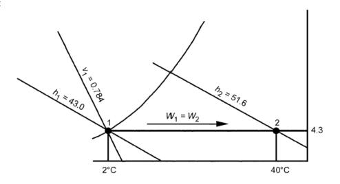
The above figure schematically shows the solution. State 1 is located on the saturation curve at 2°C. Thus,  $h_1 = 13.0 \text{ kJ/kg}$  (dry air),  $W_1 = 4.3 \text{ g}$  (water)/kg (dry air), and  $v_1 = 0.784 \text{ m}^3/\text{kg}$  (dry air). State 2 is located at the intersection of  $t = 40^{\circ}\text{C}$  and  $W_2 = W_1 = 4.3 \text{ g}$  (water)/kg (dry air). Thus,  $h_2 = 51.6 \text{ kJ/kg}$  (dry air). The mass flow of dry air is:
