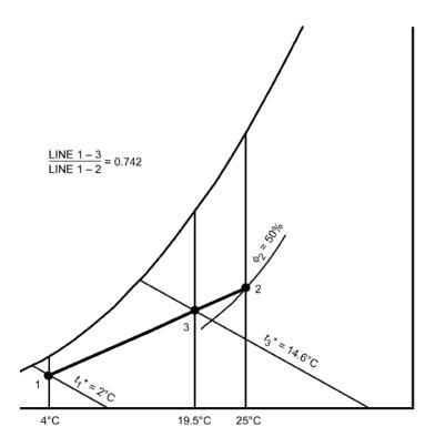
The above figure shows the schematic solution. States 1 and 2 are located on the ASHRAE chart, revealing that  $v_1 = 0.789 \text{ m}3/\text{kg}$  (dry air), and  $v_2 = 0.858 \text{ m}^3/\text{kg}$  (dry air). Therefore,
