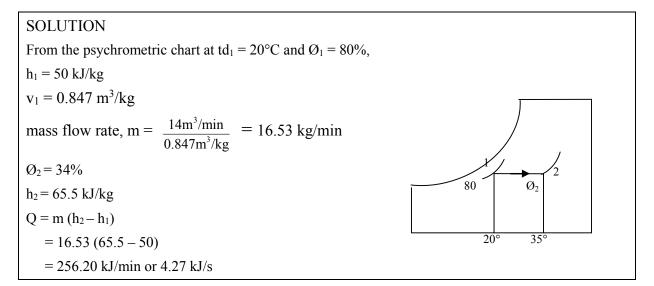
2. Determine the quantity of heat removed from 14 m<sup>3</sup>/min of air when cooled from 37°C dry bulb and 21°C wet bulb temperatures to 15°C. What are the initial and final relative humidities?
