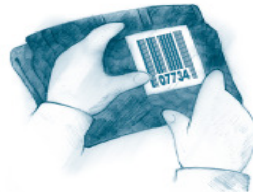
Bar codes are attached to the clothing to track it as it is assembled, washed, and prepared for shipment.
