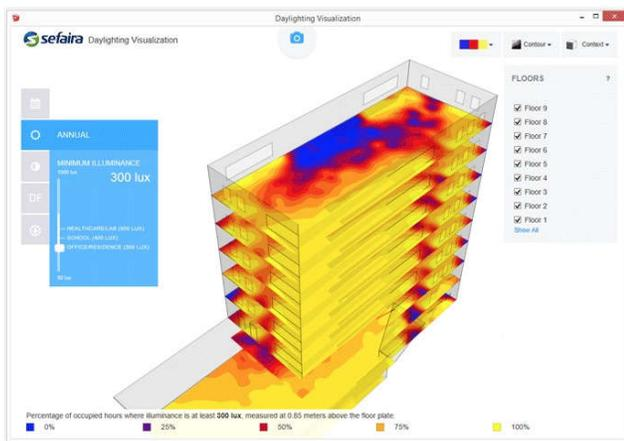
**Figure 3. BIM-supported daylight visualization and analysis** (Source: <https://architosh.com/2015/10/energy-modeling-what-you-need-to-know-about-green-building-design-and-lead/>)
