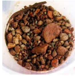
Substrate 2 (crushed brick and stones): high drainage ability, but cannot store water
