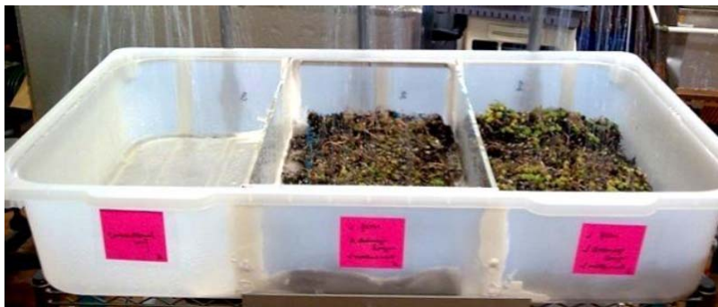
Fig. 8 Testing of modular green roof components
