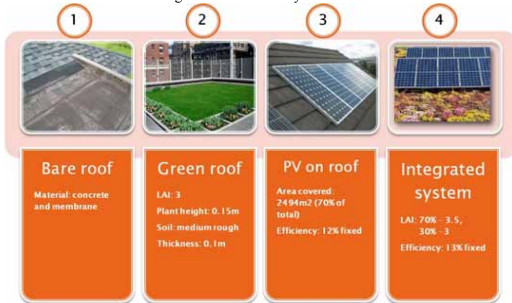
Figure 3. Four simulation models for the investigation of energy performance
