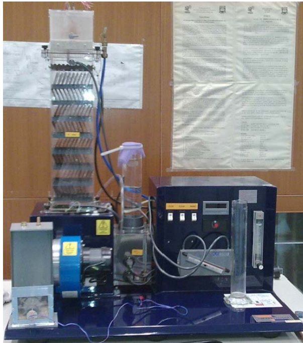
Figure 3. Cooling tower experiment unit
