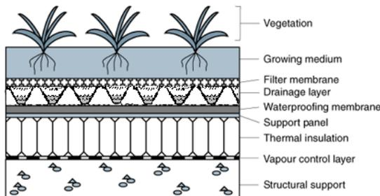
Figure 1. Typical structure of extensive green roof.
