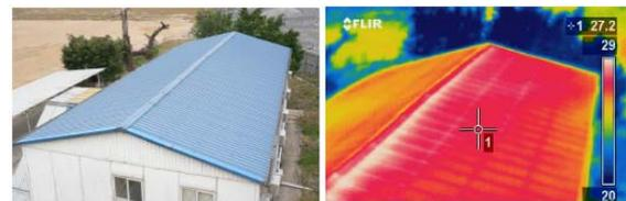
Figure 7. Infrared thermograph of a conventional roof.
