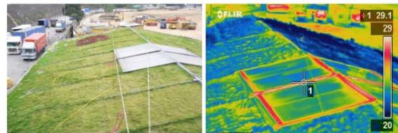
Figure 6. Infrared thermograph of the green roof.
