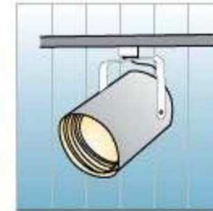
Track Lighting (Incandescent)
