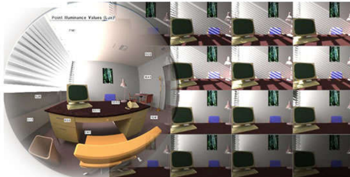
Figure 9a. A drafting office with a mirror light shelf slicing the window and redirecting light upwards.
