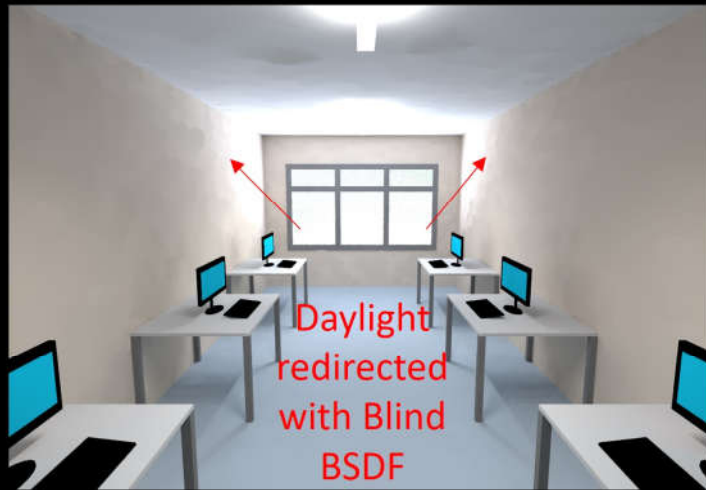
With daylight-redirecting blinds – [Uniformity = 0.31]
