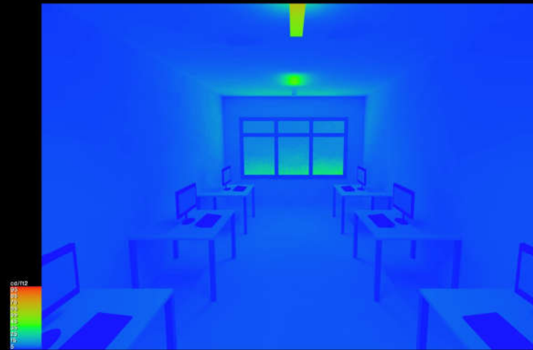
With daylight-redirecting blinds – [Uniformity = 0.31]
