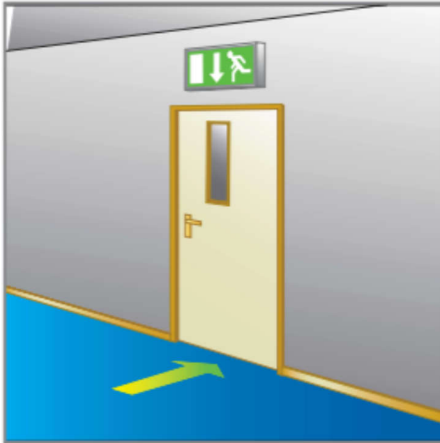
At each exit door
