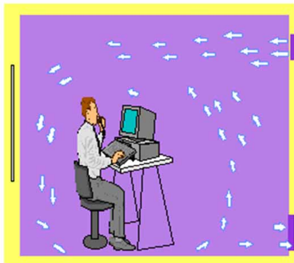
Mixing ventilation (MV)
