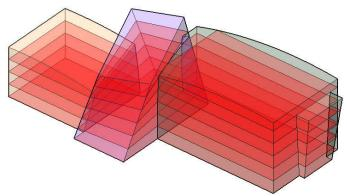
Building information modelling (BIM) can be used in conceptual design phase to explore ideas and perform early analyses for a building project. During the early planning stages of a building project, building designers can analyze the conceptual design in several ways and for various purposes. Typical studies and analyses include:
