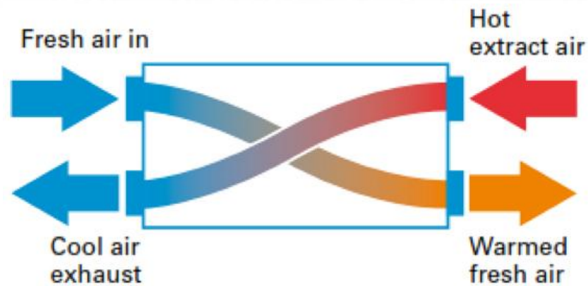
Figure 8.19 Schematic winter air conditioning system using 100 percent outdoor air with preheating by waste heat from the exhaust air.
